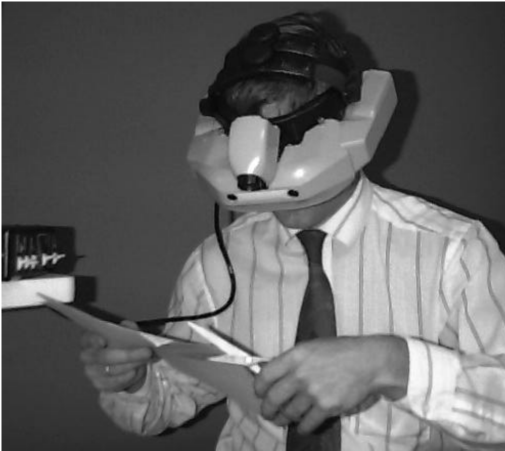
Figure 15.4 LVES wearer performing ADL. The 1995 autofocus LVES (left), allowing a patient with severe visual impairment to perform detailed visually guided activities.
